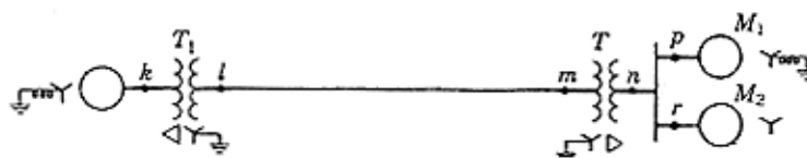
Figure 2. Power distribution system of Question 3.
