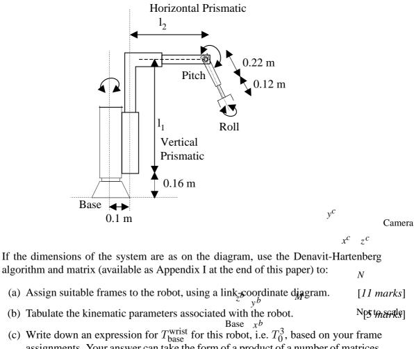
(c) Write down an expression for  $T_{\text{base}}$  for this robot, i.e.  $T_0^{\circ}$ , based on your frame assignments. Your answer can take the form of a product of a number of matrices, i.e. you are *not* required to perform the multiplication. [2 marks]
