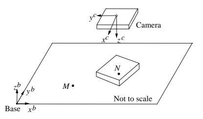
Points M and N are used for camera calibration purposes and are specified in the base frame of the robot,  $\{L_b\}$ . Points  $M^i$  and  $N^i$  are the images of M and N. The focal length of the camera is 5 cm. Note that the two test points are at different heights relative to the base. Specifically note that N has an z co-ordinate of 5 cm relative to the base.
